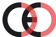
False CE Mark (too close)
